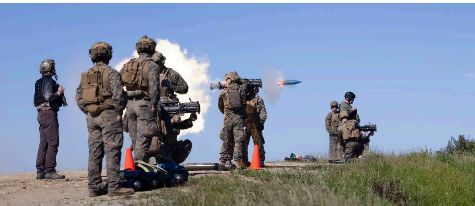
U.S. Marines with 1st Marine Division fire the M3E1 multipurpose, anti-armor, anti-personnel weapon system on Marine Corps Base Camp Pendleton, California, March 9, 2023. The MAAWS, also known as the Carl Gustaf, is a man-portable, reusable, breech-loading, 84 mm recoilless weapon system capable of destroying armored targets. (U.S. Marine Corps photo by Lance Cpl. Juan Torres)
